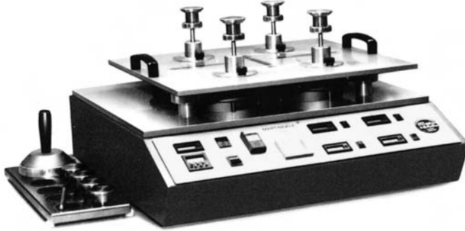
5.3 Martindale Fabric Abrasion Tester. Photograph supplied by SDL International Ltd and reproduced with kind permission.
