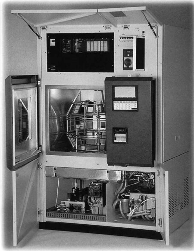
5.2 Ci4000 Weather-Ometer (Atlas Material Testing). The test samples and lamp are located in the centre of the illustration. The apparatus accurately controls the uniformity of light, temperature and humidity of the test samples. Photograph supplied by Atlas Material Testing Technology BV and reproduced with kind permission.
