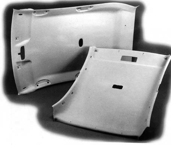
6.4 Automotive headliner covered with nonwoven fabric. Courtesy of Cosmopolitan Textile Company Ltd.
