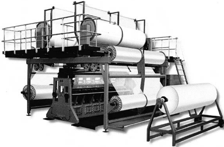
3.26 Karl Mayer double-needle-bar knitting machine RD6 DPLM – front view. (Reproduced by kind permission of Karl Mayer Textilmaschinenfabrik GmbH.)
