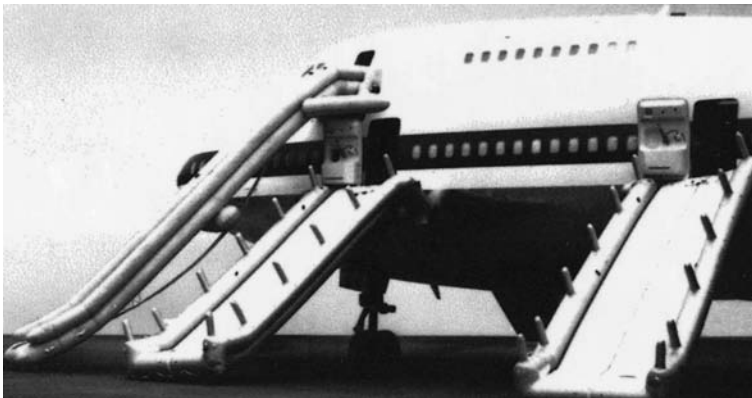
9.6 Aircraft evacuation slide. Reproduced with kind permission of Reeves Brothers, Inc.
